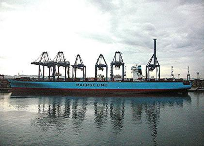
was still going on. Since the containers were being put below deck we couldn't see the progress that had made. In the photo on the left the second and forth cranes from the left have empty container grippers returning to the dock for reload while the fifth crane has a container being lowered into the ship's hold. Finally, about 5pm the forward hold apparently was filled and, as shown in the photo on the left,
